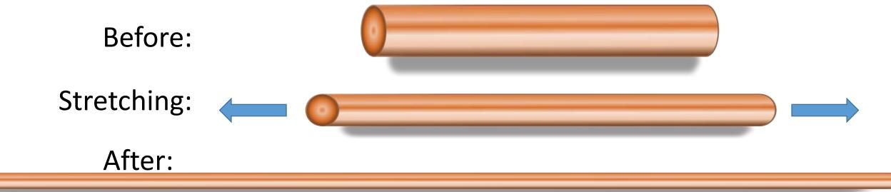
Constraint: Tension Deformation: Plastic
